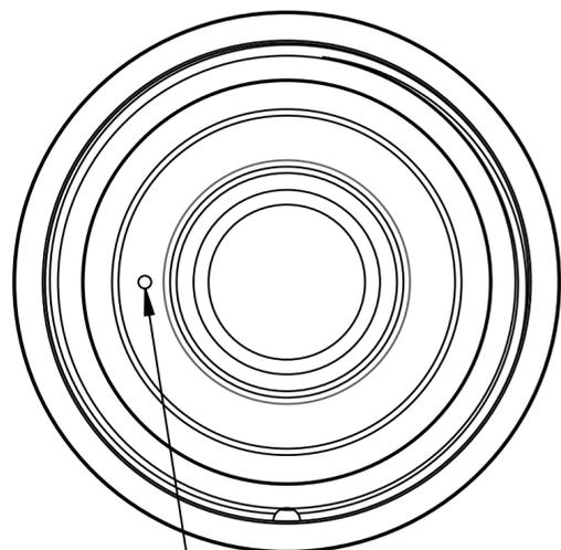
A MINIMUM OF ONE DOT WILL BE PRESENT AS IDENTIFYING MARK FOR "BEARING HOUSING: DHX2, U-CUP, 14X4mm GLAND"
