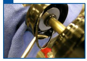
Replace the backup ring, seal, backup ring, and dust wiper into 21 the air sleeve seal glands. Tip: Squeeze the backup ring like a "potato chip," as shown, to facilitate installation.
