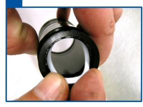
Place 2cc of FLOAT Fluid into the air sleeve. Do not screw the 23 air sleeve on at this time.
