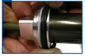
If necessary, remove the air sleeve dust wiper, seal and backup 20 rings. Carefully remove these parts using a dental pick. If you
