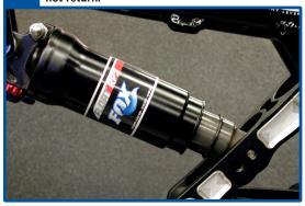
O3 The shock may extend slightly. However, the shock can still be "stuck down." Continue on to the next step with caution.
