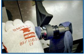
11 Remove the shop towel from the body eyelet then fully remove the air sleeve.
