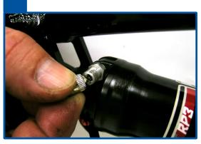
**06** Remove the mounting hardware and remove the shock from the bicycle. In most cases, a hex wrench is all that is necessary to remove the mounting hardware. Hex wrench size will vary depending on manufacturer.
