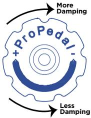
The ProPedal adjustment knob allows the rider to adjust the amount of ProPedal damping. ProPedal damping affects the first part of the compression stroke and is designed to control pedal-induced suspension bob. Since suspension designs vary, not all bicycles require the same degree of ProPedal damping provided by the Boost Valve.
